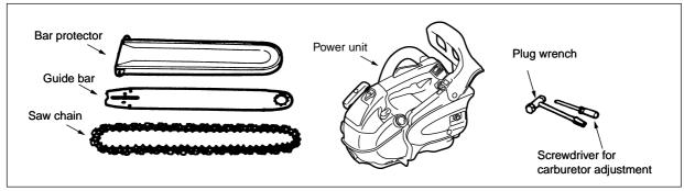
Open the box and install the guide bar and the saw chain on the power unit as follows:
